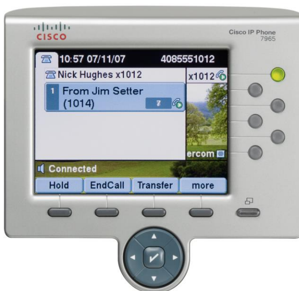
Figure 2. Close-Up of Display and Lighted Line Keys
